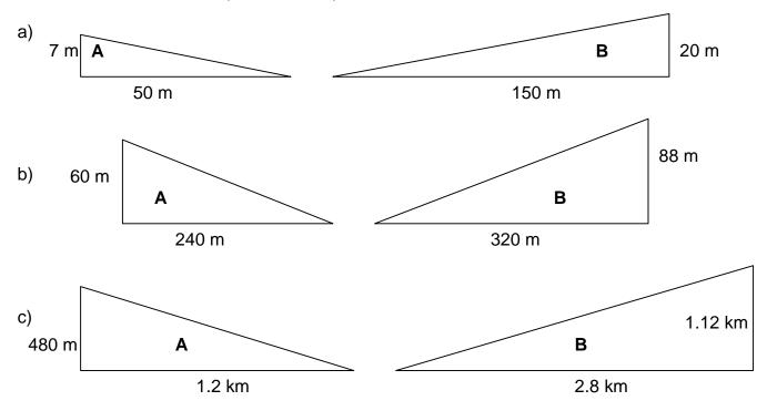
3. A wheelchair ramp is to be built. Guidelines state that the ramp must have a gradient of less than 0.3. Does the plan below fit the guidelines – justify your answer.
