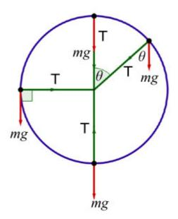
Consider a mass m performing circular motion under gravity, the circle with radius r. The centripetal force on the mass varies at different positions on the circle.
