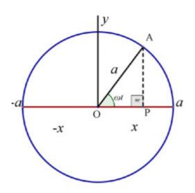
The SHM-circle connection is used to solve problems concerning the time interval between particle positions.
