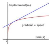
For a displacement-time graph, the gradient at a point is equal to the speed.
