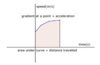
For a speed-time graph, the area under the curve is the distance travelled.
