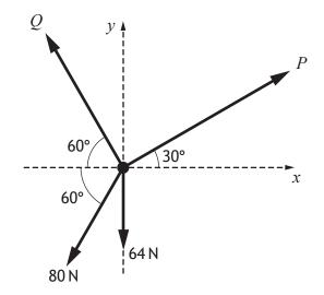
The tensions in the four ropes are P, Q, 80 and 64 newtons respectively, and their directions relative to the axes are shown.
