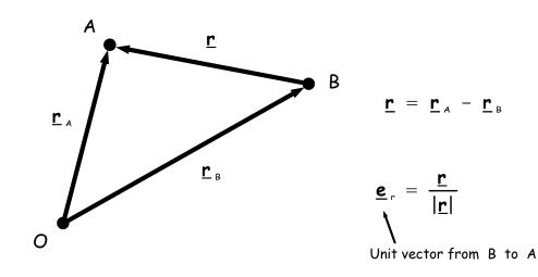
The gravitational force exerted on A due to B, denoted by  $\mathbf{\underline{F}}_{AB}$ , acts along the vector  $-\mathbf{\underline{r}}$  from A to B and is given by,
