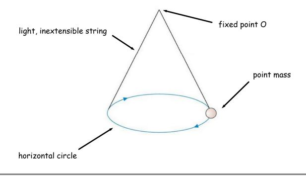
In a conical pendulum, there are always two forces that act on the point mass (aka bob): string tension and gravity.
